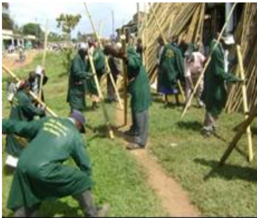
Plate 3: Farmers scraping bamboo and removing nodes
