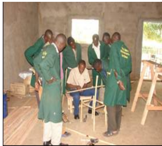
Plate6: Trainer demonstrating on bamboo chair frame making
