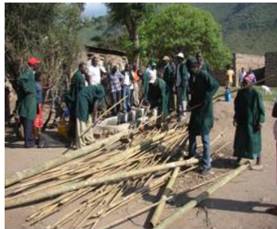
Plate 2: Farmers arranging bamboo in the bamboo treatment trench
